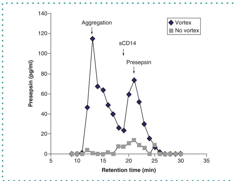
**Figure 1.** Size exclusion chromatogram of plasma before and after agitation. The presepsin concentration of plasma was determined by PATHFAST-Presepsin. Plasma (before and after vortex) were applied and eluted with PBS containing 0.05% Tween-20 on Sephadex G75 10/300 column and the presepsin concentrations of each fraction were determined. The peak of sCD14 was founded by CD14-ELISA (R&D systems, MN, USA). sCD14: Soluble CD14.
