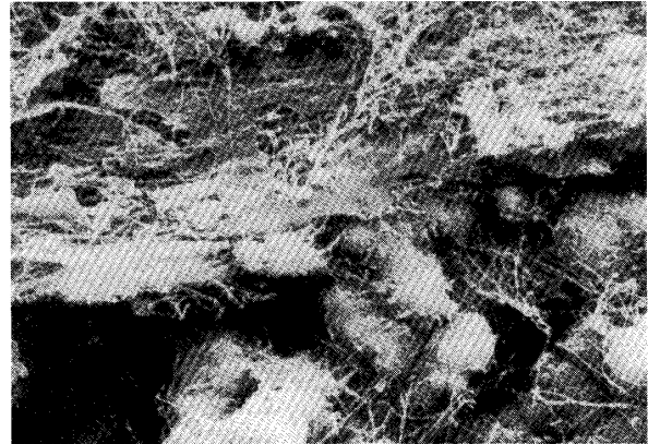
Fig. 16. Scanning electron micrograph of the anodic oxidation-hydrothermal treated hydroxyapatite coating titanium surface after 14-days-culture ( \times 15000 ). The calcified-like microspheres and network of collagen-like fibers at the surface of anodic oxidation-hydrothermal treated hydroxyapatite coating titanium (from reference 17)
