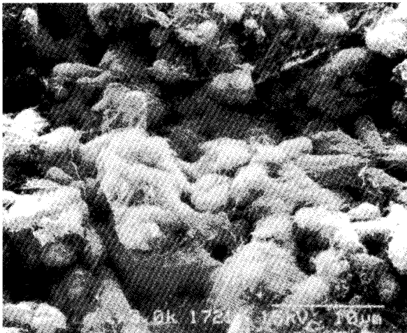
Fig. 15. Scanning electron micrograph of the anodic oxidation-hydrothermal treated hydroxyapatite coating titanium surface after 14-days-culture ( \times 15000 ). The calcified-like microspheres at the surface of anodic oxidation-hydrothermal treated hydroxyapatite coating titanium (from reference 17)
