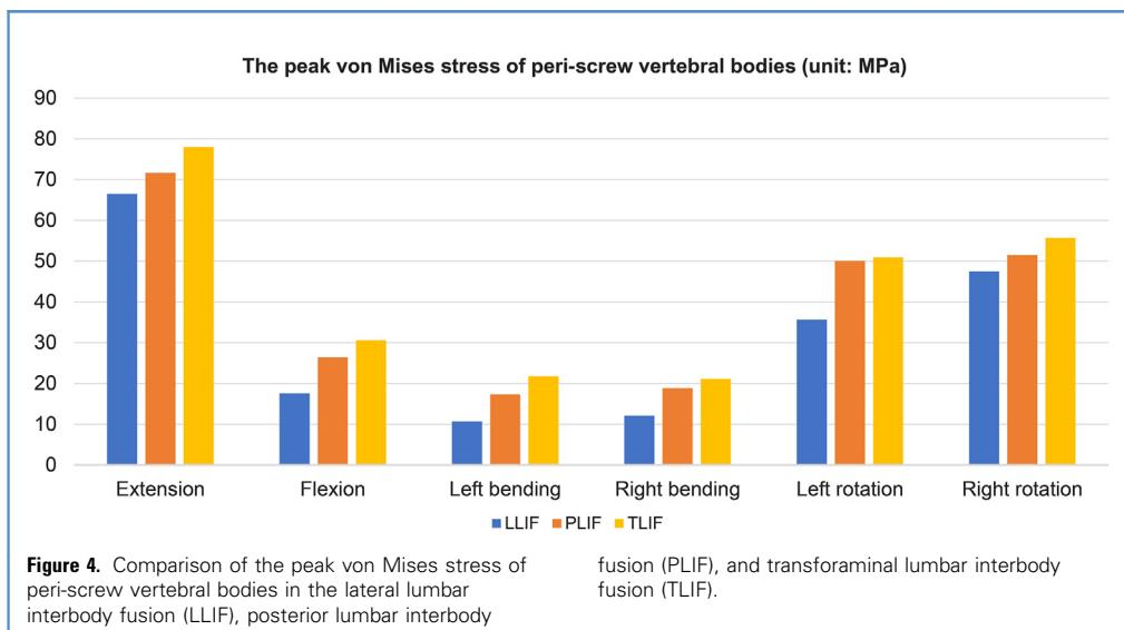
**Figure 4.** Comparison of the peak von Mises stress of peri-screw vertebral bodies in the lateral lumbar interbody fusion (LLIF), posterior lumbar interbody fusion (PLIF), and transforaminal lumbar interbody fusion (TLIF).
