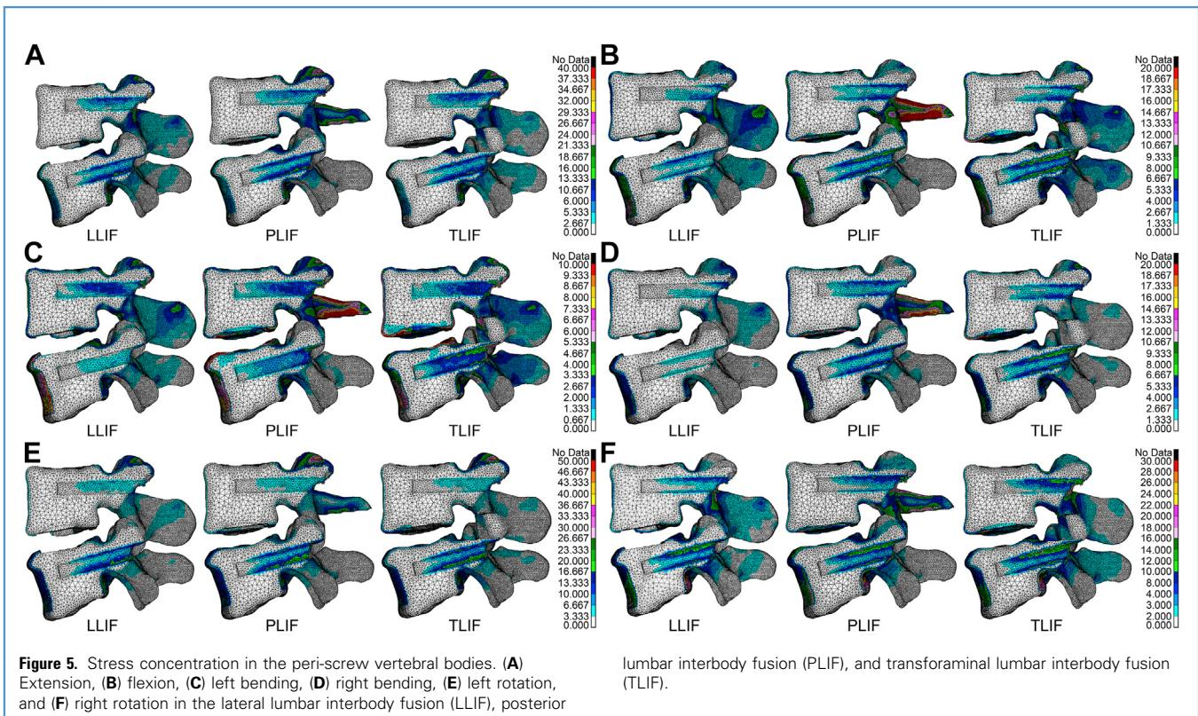
**Figure 5.** Stress concentration in the peri-screw vertebral bodies. (A) Extension, (B) flexion, (C) left bending, (D) right bending, (E) left rotation, and (F) right rotation in the lateral lumbar interbody fusion (LLIF), posterior lumbar interbody fusion (PLIF), and transforaminal lumbar interbody fusion (TLIF).
