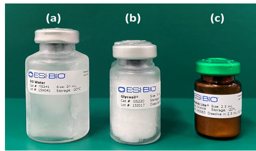
Figure 2. A cross-linkable hyaluronic acid kit, Hystem ® , consisting of: (a) degassed (DG) water; (b) hyaluronic acids possessing –SH functional groups (Glycosil ® ); and (c) thiol-reactive polyethylene glycol diacrylate (PEGDA) cross-linker (Extralink Lite ® ).
