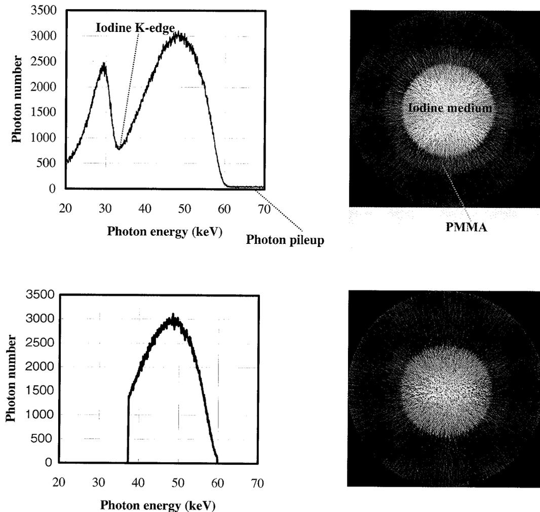
Fig. 4. X-ray spectra and tomograms of a PMMA phantom filled with iodine contrast medium with an iodine density of 35 mg/mL (a) using a photon energy range from 20 to 60 keV and (b) a range from 37 to 60 keV.
