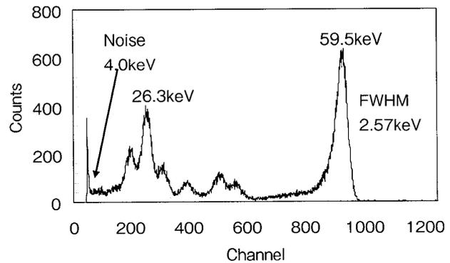
Fig. 3.  $\Gamma$ -ray spectra from an Am241. The channel number is proportional to the photon energy mostly.
