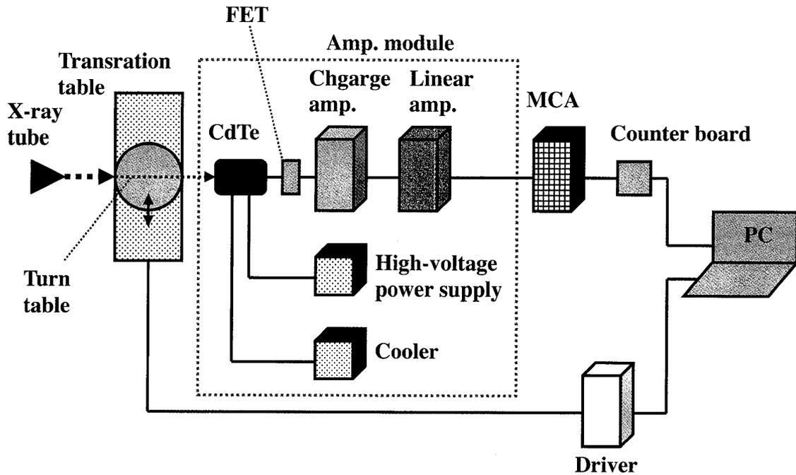
Fig. 1. Block diagram of a photon-counting x-ray CT system utilizing a CdTe detector.
