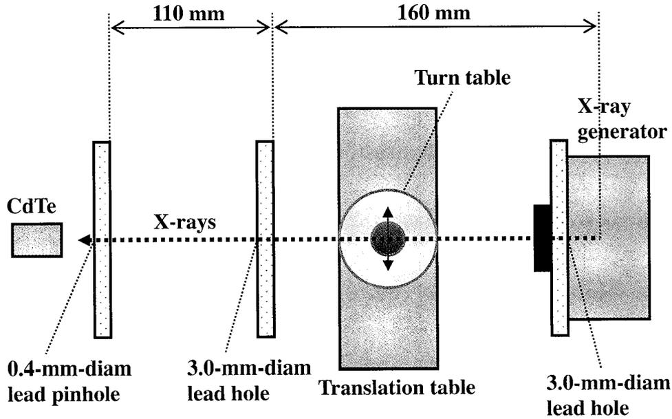
Fig. 2. Experimental setup for photon counting.
