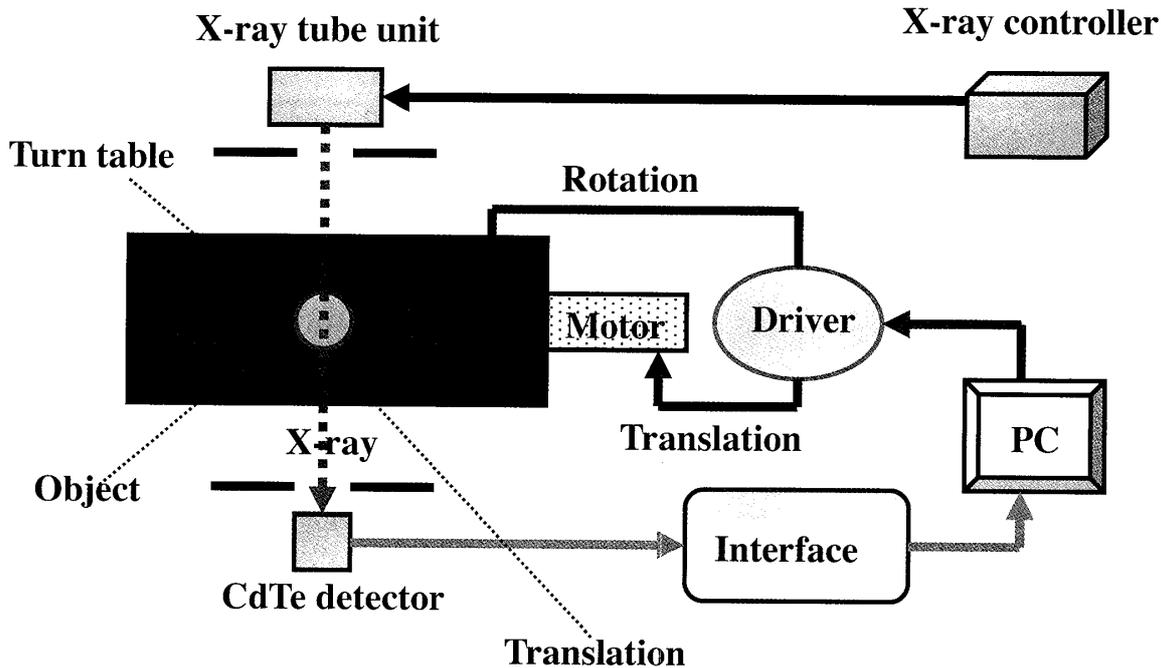
Fig. 1. Block diagram of a simple x-ray CT system utilizing a CdTe detector.
