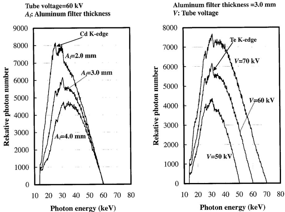
Fig. 3. X-ray spectra from the generator (a) according to changes in the aluminum filter thickness at a constant tube voltage of 60 kV and (b) changes in the tube voltage using a 3.0-mm-thick aluminum filter.
