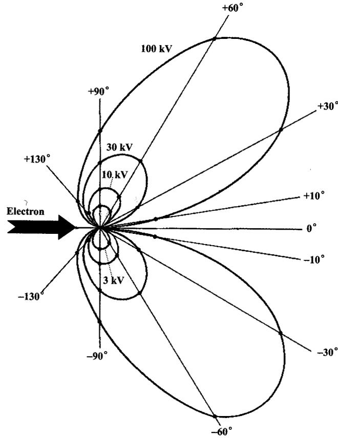
Fig. 5: Bremsstrahlung x-ray distribution with the angle.
