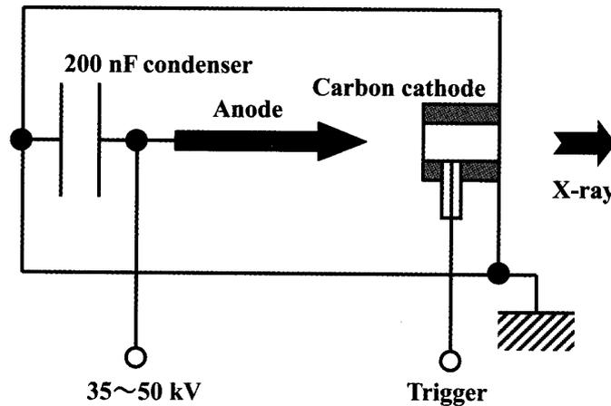
Fig. 2: Circuit diagram of the plasma x-ray generator.
