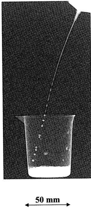
Fig. 11: Radiogram of water droplets falling into a polypropylene beaker from an injector.
