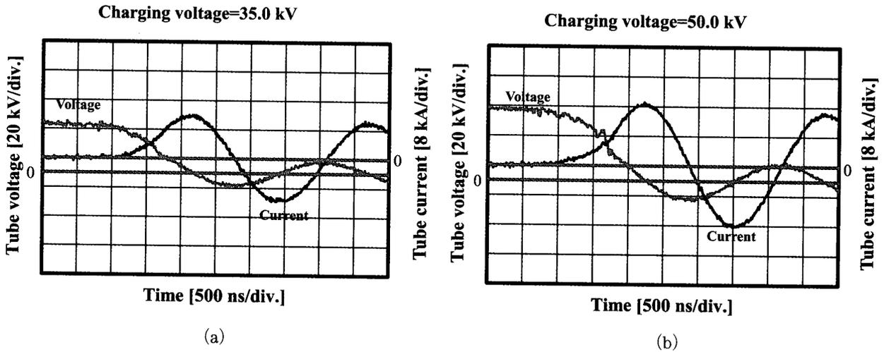
Fig. 6: Tube voltages and currents with a charging voltage of (a) 35.0 kV and (b) 50.0 kV.
