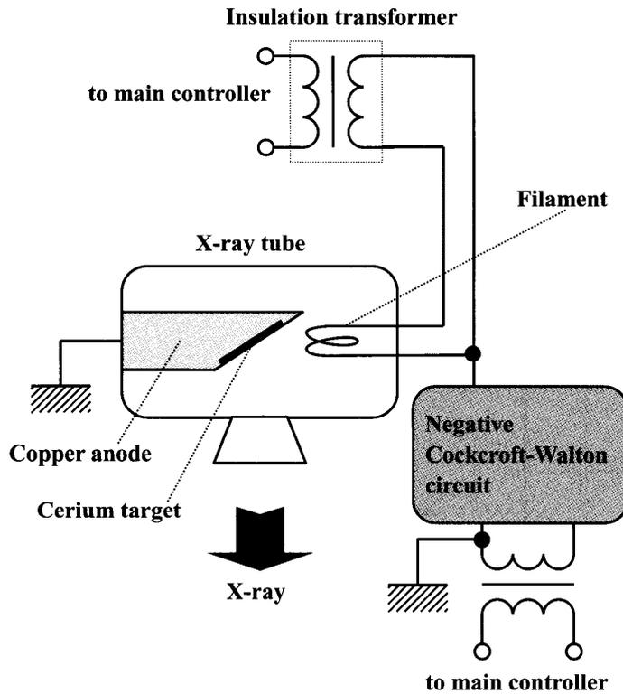
Fig. 4: Main circuit of x-ray generator.
