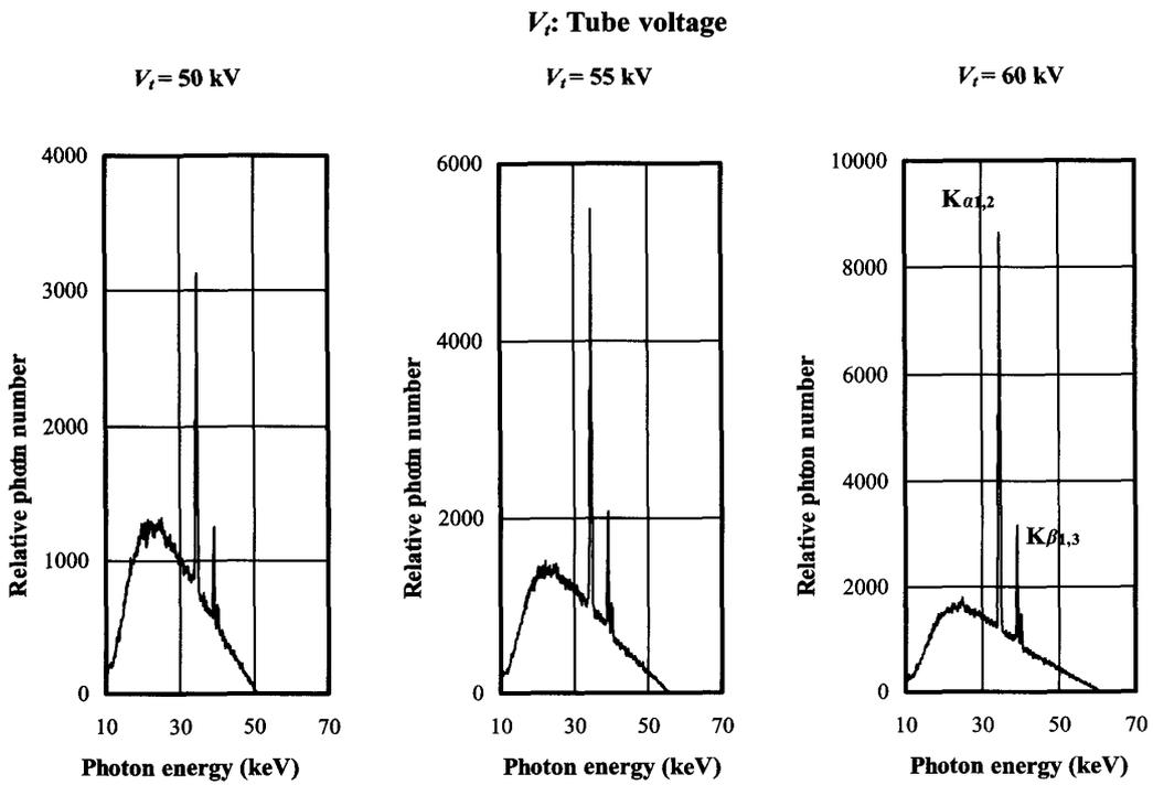
Fig. 7: X-ray spectra measured using germanium detector.
