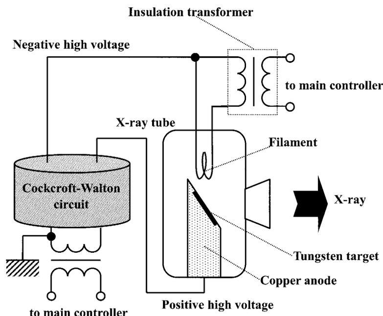
Fig. 2: Main circuit of the x-ray generator.
