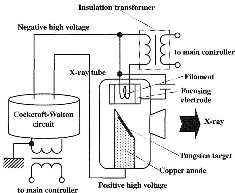
Fig. 1. Electric circuit of the x-ray generator.
