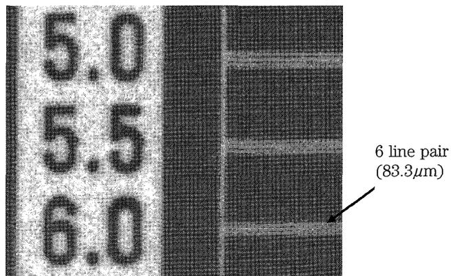
Fig. 4. Radiograms of a test chart for measuring the spatial resolution.
