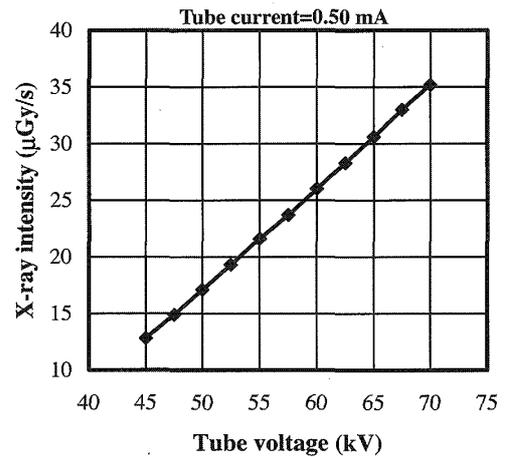
Fig. 2. X-ray intensity ( $\mu\text{Gy/s}$ ) as a function of tube voltage (kV) with a tube current of 0.50mA.
