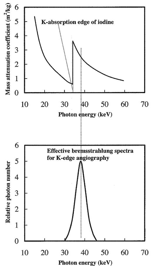
Fig. 6. Mass attenuation coefficients of iodine and effective bremsstrahlung x-rays for enhanced K-edge angiography.
