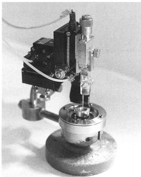
Fig.2 Photograph of the microdrive.
