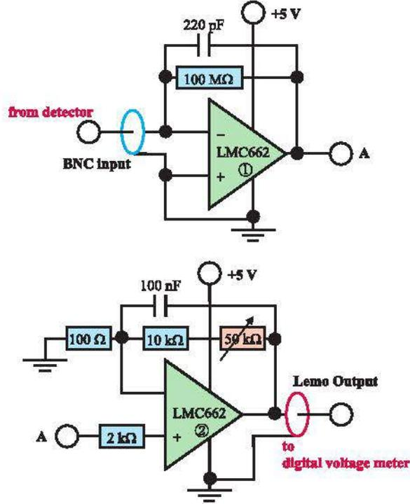
Fig. 3. Circuit diagrams of I-V and V-V amplifiers in the X-ray detecting module.
