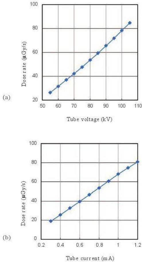
Fig. 4. X-ray dose rate measured using an ionization chamber placed 1.0 m from the X-ray source. (a) Tube voltage dependence at a tube current of 0.8 mA, and (b) tube current dependence at a tube voltage of 80 kV.
