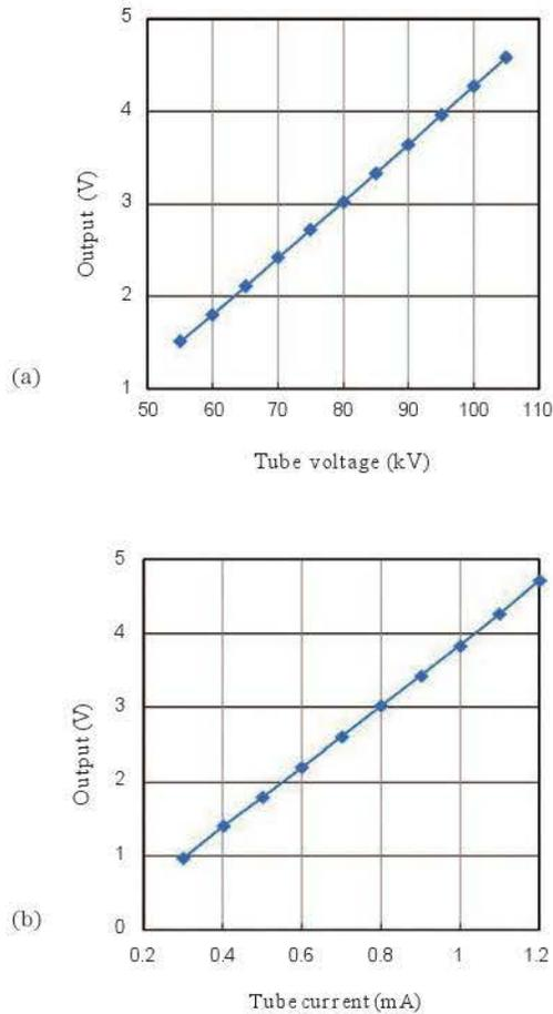
Fig. 5. Output voltages from the module. (a) Variations with the tube voltage at a tube current of 0.8 mA, and (b) variations with the tube current at a tube voltage of 80 kV.
