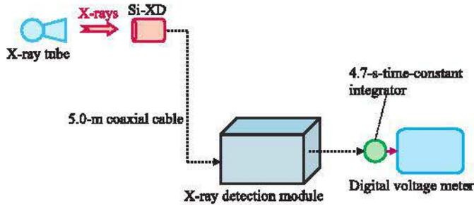
Fig. 1. Block diagram for detecting low-dose-rate X-rays using a Si-XD, a 5.0-m coaxial cable, an X-ray detecting module, and an X-ray generator. The Si-XD is placed 1.0m from the X-ray source, and the output voltage is measured using a digital voltage meter with an integrator.
