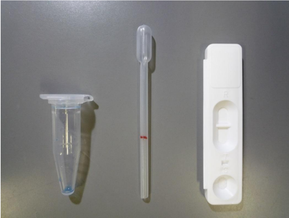
Figure 1 A microtube containing blue pretreatment liquid (left), a dropper that has a red line on it (middle), and the main unit of the kit (right).
