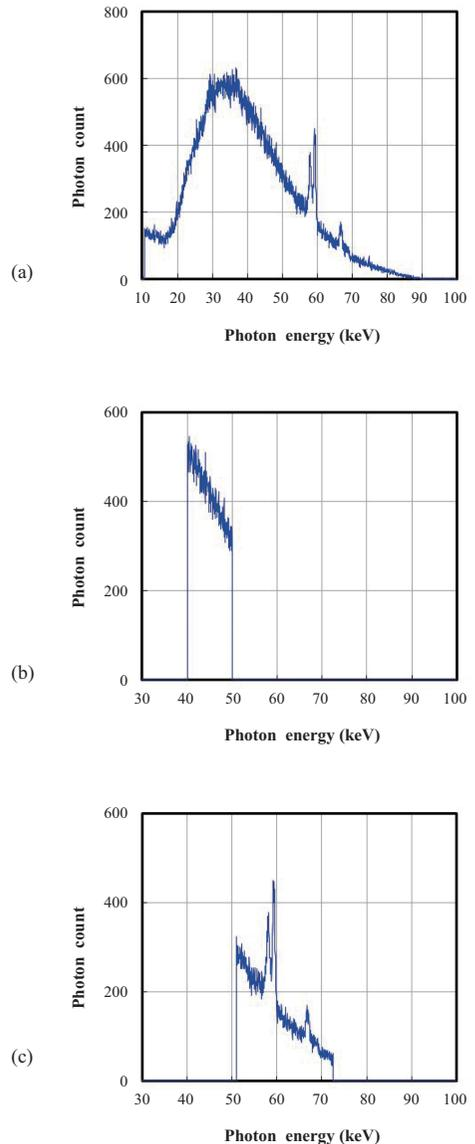
Fig. 5. The X-ray spectra measured using the CdTe detector in the quasi-monochromatic ED-CT system. (a) Entire spectra with energies ranging from 10 to 90 keV, (b) discriminated photons with energies ranging from 40 to 50 keV, and (c) discriminated photons with energies ranging from 50 to 72 keV for Gd-K-edge CT.
