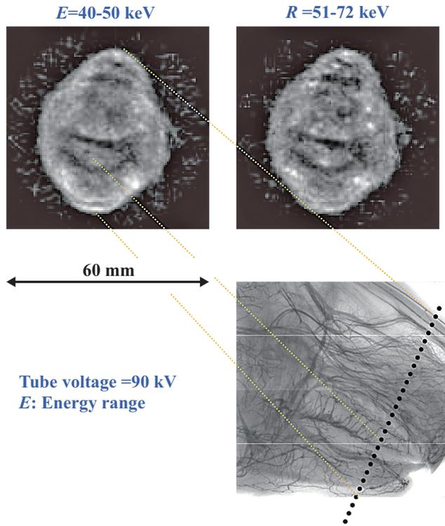
Fig. 8. Tomograms of a rabbit-head phantom. Blood vessels were filled with Gd-based microparticles.
