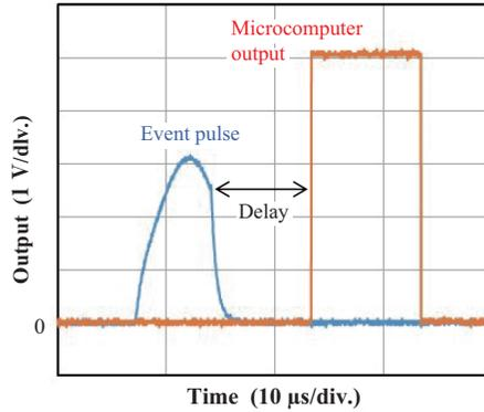
Fig. 6. Time relationship between the event-pulse and the MC outputs.
