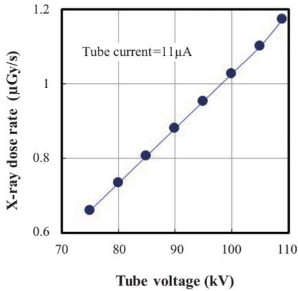
Fig. 4. X-ray dose rate measured at 1.0 m from the X-ray source and a tube current of  $11 \mu\text{A}$ .
