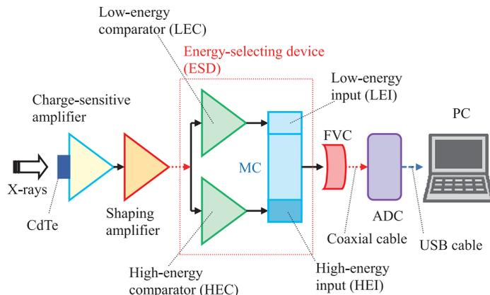
Fig. 1. Block diagram for counting quasi-monochromatic X-ray photons using a CdTe detector and an ESD. The ESD consists of a LEC, a HEC, and an MC.
