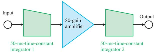
Fig. 2. Block diagram of the FVC. The logical pulses from the MC are converted into long-pulse voltages and piled up in the first integrator, and the integrator output is amplified by a V-V amplifier. The second integrator is used to reduce the electric noises.
