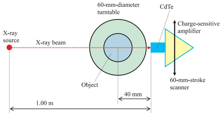
Fig. 3. Experimental setup of the main components in the quasi-monochromatic ED-CT system. The ED-CT is performed by repeated linear scans and rotations of the object.
