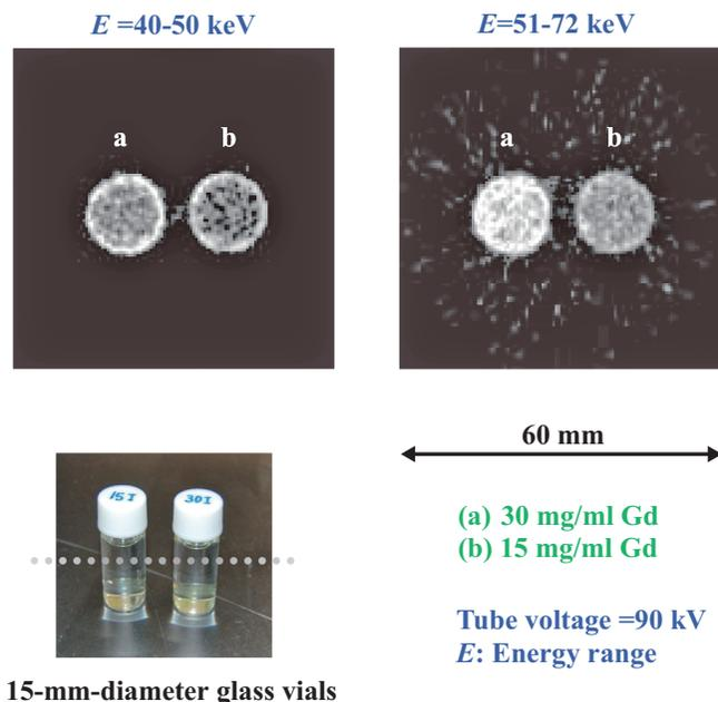
Fig. 7. Tomograms of two glass vials filled with Gd media of two different densities of 15 and 30 mg/ml.
