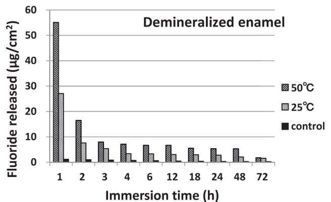
Fig. 3 – Amount of  $F^-$  released from demineralized enamel surface with APF applied. Longer lasting and greater amounts of  $F^-$  release were observed in the demineralized specimens than in the sound specimens. Both the 50 °C group and the 25 °C group showed significantly greater amounts of  $F^-$  release than control up to 72 h. Also the significant differences were observed between the 50 °C group and the 25 °C group up to 48 h.
