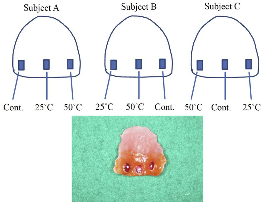
Fig. 1 – Photograph and schematic diagram of the intraoral device for *in situ* experiments. Three shallow dents were made on the palatal surface and a demineralized specimen in each group was mounted with sticky wax. They were mounted systematically by shifting the specimen position to randomize the potential influence by  $F^-$  contamination released from the neighboring specimens.
